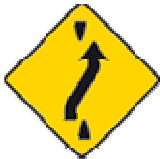
Traffic cross-over ahead
